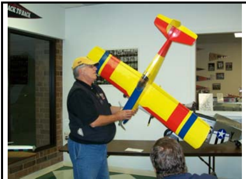
Harlan Davis's Sig Four Star built from a kit with a 40 size engine.
